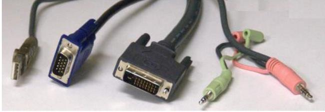
Figure 3. Cable connectors to the personal computer. You will need to connect one of the video ports (DVI or VGA) and the USB cable. If you want to play any sound, you will also need to connect the green connector (🔊) to your audio output port. If you want to record speech to your computer, you will need to connect the pink connector (🎤) to your microphone port. Note that the audio port and microphone port have the same size, so you will need to distinguish them by color or symbols.
