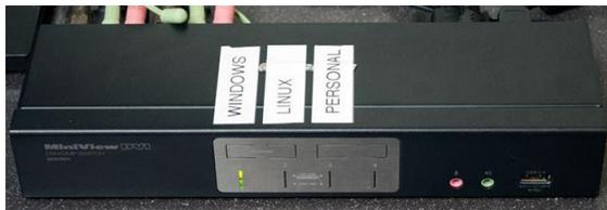
Figure 4. Four-channel KVM switch. This is the switch to select different stimulus computers. It will switch video, audio output, microphone input and USB to one of the stimulus computers.
