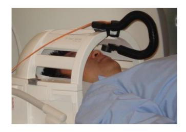
Figure 9. Speech recording microphone, the flex-boom and stand to mount it to the subject. The microphone should be as close to the subject's mouth as possible, but without touching subject.
