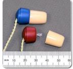
Figure 7. HiFi earphones and the earplugs. Red one is right channel and blue one for left channel (you can remember this by two R's: red for right). The earplugs are screwed on the plastic tubes.
